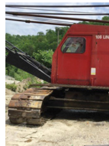
GRUA LINK BELT LS108 40 TON Cap: 40 Tons Pluma: 18m
