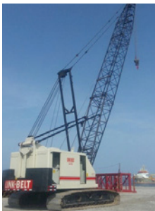
GRUA LINKBELT 318 80 TON Cap: 80 Tons Pluma: 36m
