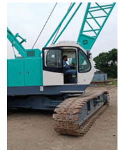
GRUA KOBELCO 70HD Cap: 70 Tons Pluma: 32m
