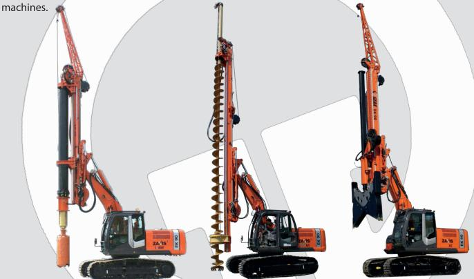
The GEAX EK90 (in common with other GEAX machines) has an articulation structure similar to a normal excavator with a long boom supporting the mast. This allows a wide range of mast positioning and independent adjustment of the vertical position of the mast. Wire rope positions are not dependent on the position of the mast as the winches are mounted on the mast itself. This design, compared to other machines, usually with parallelogram type mast supports, ensures the following:
