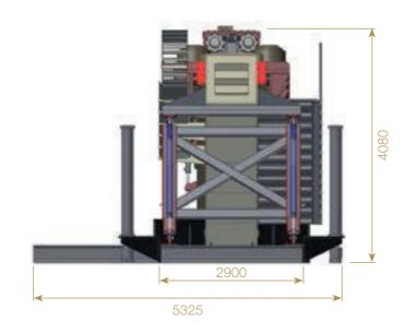
THDD 450 Horizontal Directional Drilling Machine with 450 tons pulling capacity is the first in Turkey and one of the leading in the world manufactured by Özkanlar Machinery.
