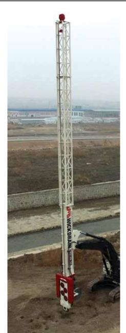
The OMS Wick Drain Insert Machine is a soil improvement machine that to be used for quick consolidation of the cohesive soils. The machine is consisting of; hydromotors, sprocket gears, mandrel and a high frequency vibro hammer. It is very useful equipment to drain the water in the cohesive soils, thus, the liquefaction risk minimal and settlement time higher then standard procedures.
