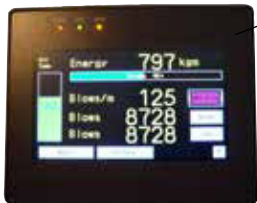
INTERFACE SCREEN MOUNTED ON POWER PACK
